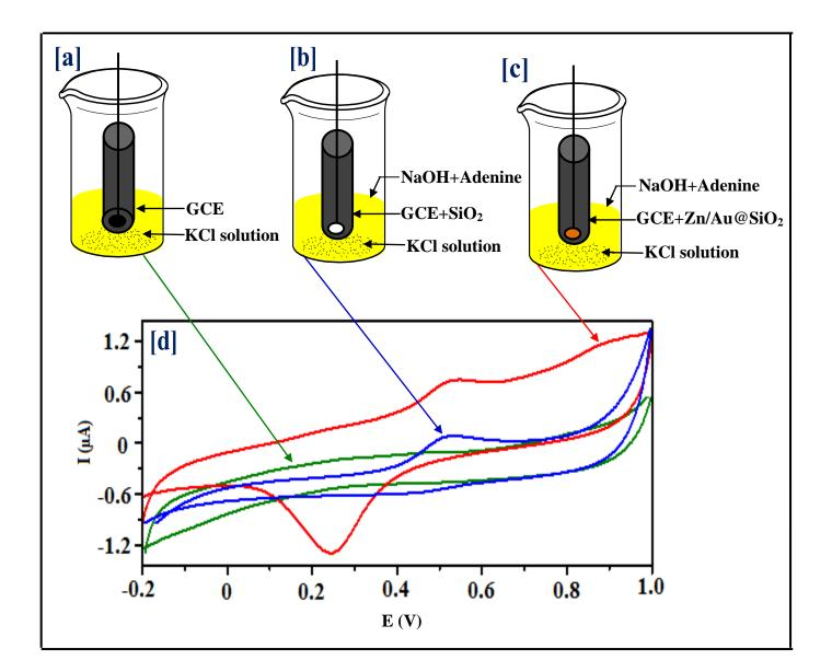
Figure 2. CVs of uncoated GCE with 0.2 M KCl solution (green curve),  $SiO_2$  coated GCE in 0.2 M KCl with 0.002 M Adenine solution (blue curve) and Zn-Au@SiO<sub>2</sub>coated GCE in 0.2 M KCl with 0.002 M Adenine solution (red curve).
