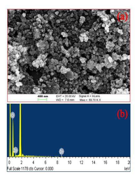
Figure. 1 (a) SEM image of Zn-Au@SiO<sub>2</sub>nanoparticles and (b) EDX analysis of Zn-Au@SiO<sub>2</sub>.
